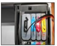
Open the cover for the cartridges
