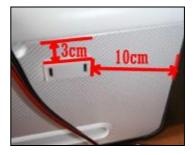
Slightly press every cartridges to check all the cartridges are in the correct position. And Please be care about the tubes which out through the box .Then stick the Support Arm on the Position which show in the third picture.
